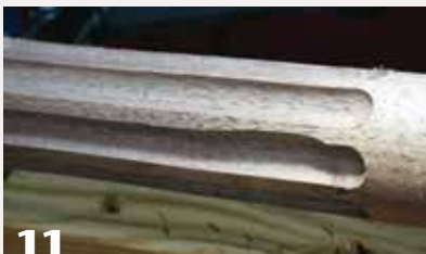
11 Plunging the full diameter of the router bit into the wood will cause the router to ride upward, so keep steady downward pressure on the router.
