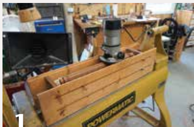
1 The author's first attempt at using a router on turned items involved a box that held the workpiece and guided the router.
