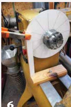
(6) A simple shopmade indexing wheel with marked positions and a rudimentary but effective locking mechanism—a spring clamp.
