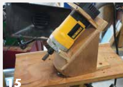
15 Positioning the router at an angle to the workpiece offers some advantages and increased design opportunities.
