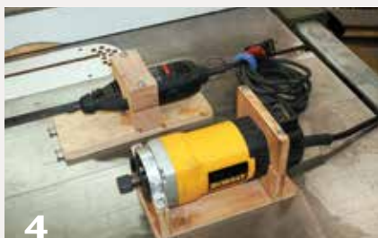
4 There are various ways to secure the router (or rotary tool) to a wood base, including wood blocks and aluminum strapping.
