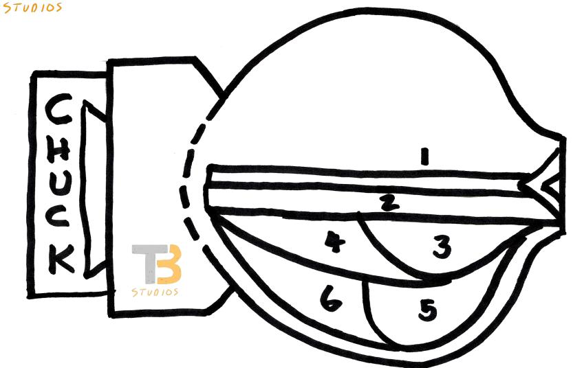
STEP 1: BORE A HOLE TO DEPTH
