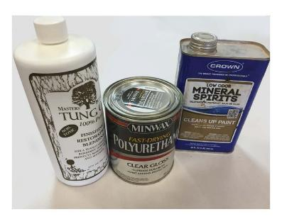
The oil/varnish I use is a mix of 1/3 pure Tung oil, 1/3 gloss polyurethane, and 1/3 mineral spirits. I apply it with a paper towel, making sure to wipe off any excess.
