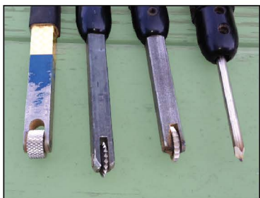
Detailing Tools: Knurling, texturing, spiraling and Pyramid.
